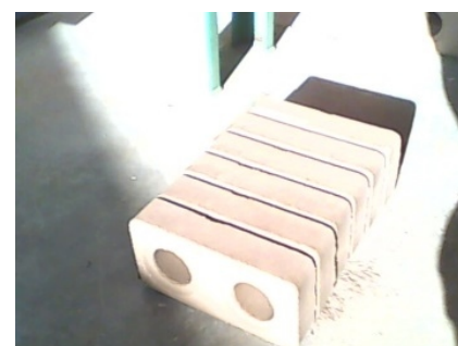
Figure 15. Sludge from water treatment plant-coal fly ash-soil-cement bricks.
