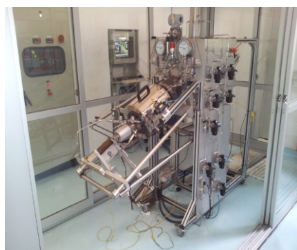
Figure 11. Batch reaction system microwave-assisted and conventional heating.
